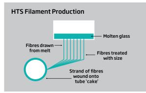
producing high tensile strength glass fibre filament.
